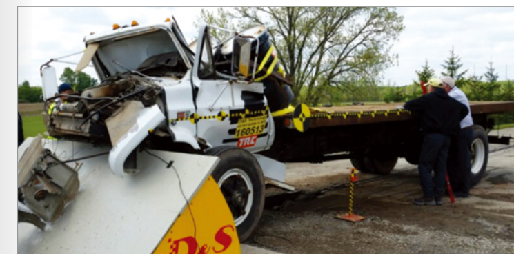
[Collision Test: Completely blocked 6.8 t truck moving at 80 km/hr]
