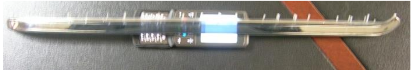
↑ HMC IP-GARNISH Half Mirror VM (Transparent Rate 7%, AL VM)
