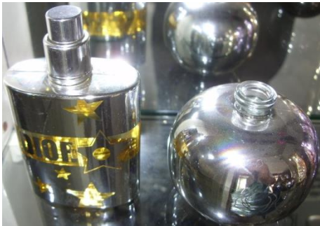
↑ Perfume bottle Metallizing with Laser or Print (Amore Pacific)
