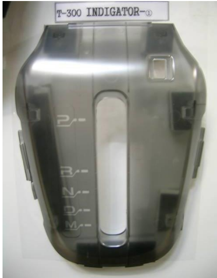
↑ HMC IP-GARNISH Half Mirror VM (Transparent Rate 7%, AL VM)
