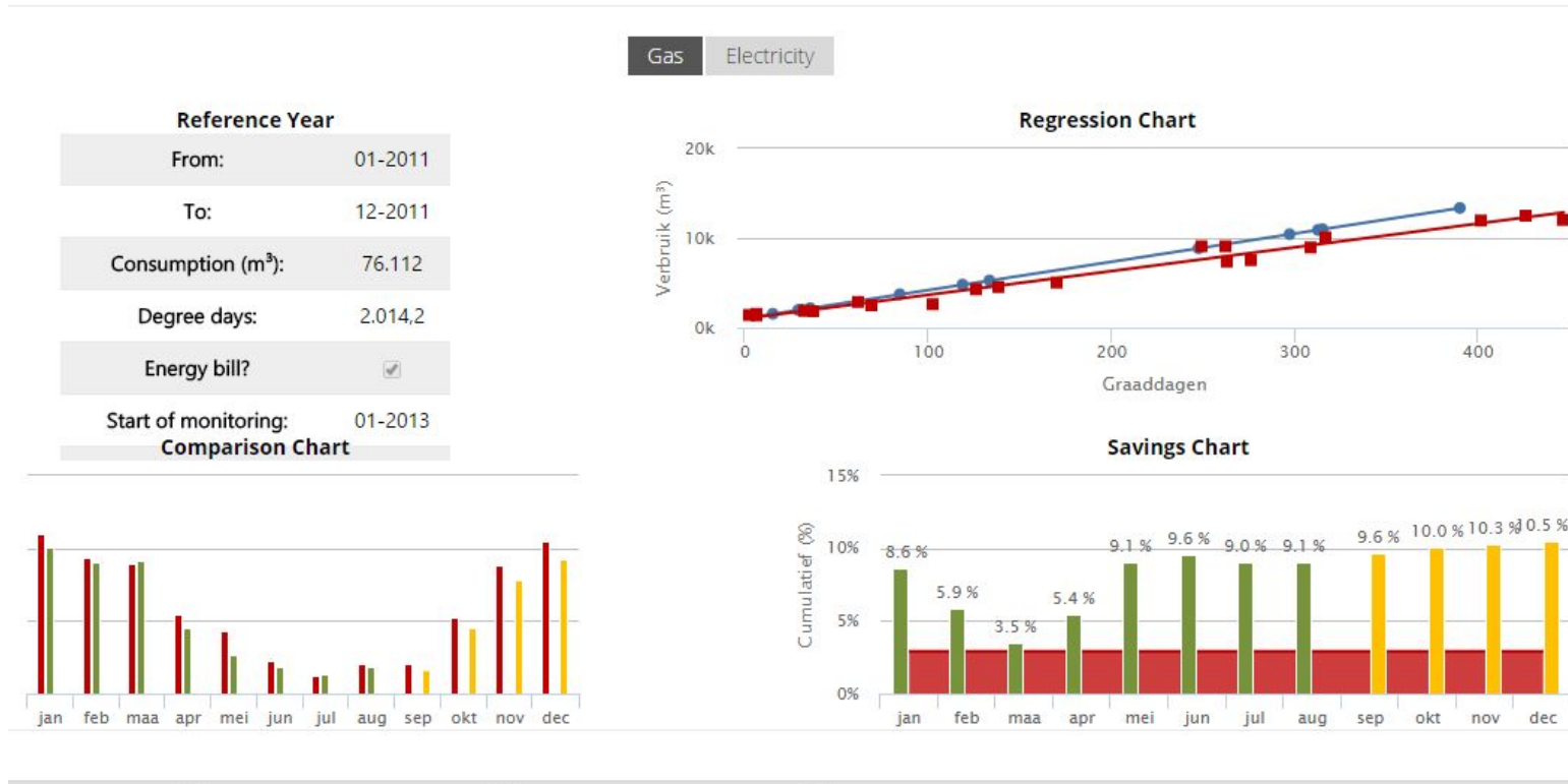
Fig 13 - Monitoring the progress
